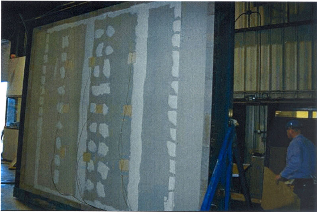
Figure B-3. Unexposed Side of the Wall With Instrumentation is Completed.
