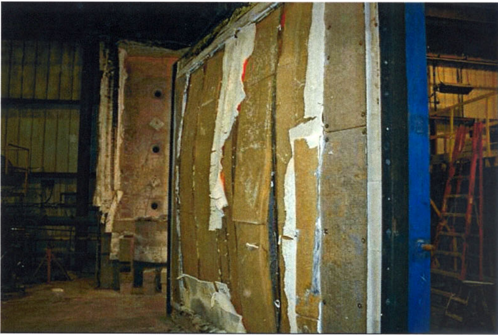
Figure B-9. Exposed Side of Wall Assembly After the Fire Test.
