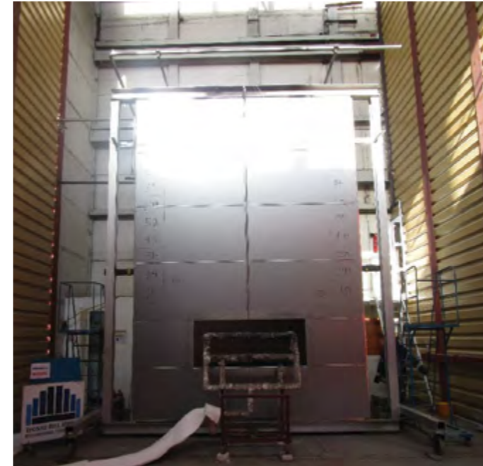
EXTERIOR FACE PRIOR TO FIRE TEST.
