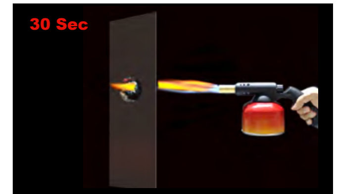
Solid Aluminium Panel Fire Penetrated In 30 Seconds
