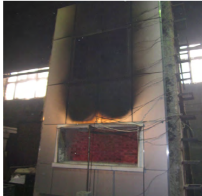
FIRE STOPPED AFTER 60 MINUTES ALL PANELS WITHOUT DAMAGE
