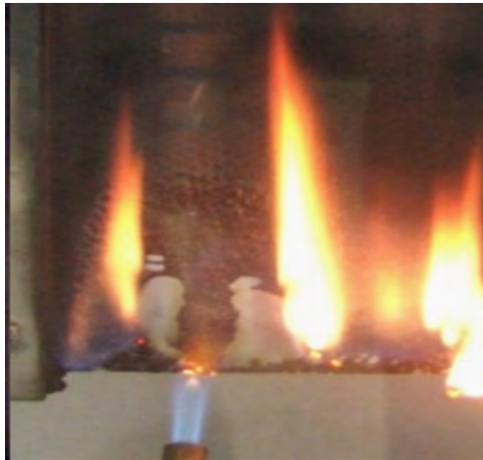
EN 13501 PART THREE : Small flame attack
