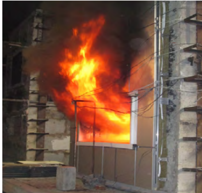
FULL FIRE IN BOTH FLOORS - TEMPERATURE 850 °C
