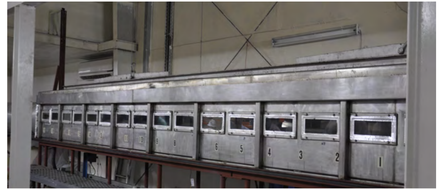
Steiner Tunnel Fire Machine
