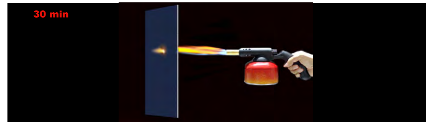
A2 MINERAL CORE - ACP PANEL - Fire Penetrated In 30 Minutes
